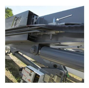
Move the pressure gauge to the HOP manifold and install it on port G2. With the unit running check the reduced/pilot pressure. Set this pressure to 350 psi using the pressure reduced (PR) cartridge.
