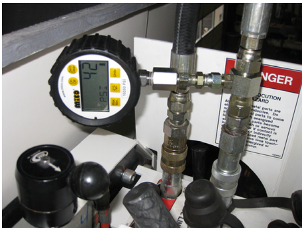
TESTING FOOT VALVES
