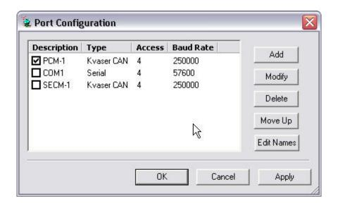
The Baud Rate for the PCM-1 port needs to be set to 500000 to correctly communicate with the HyPowerTM system. To edit the PCM-1 port, click on the PCM-1 description to highlight it and then click on Modify.
