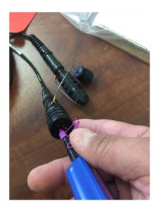
If the connection issue still exists and the battery has been replaced, the issue is with the lower fiber optic receiver, upper fiber optic receiver, or the fiber optic cable.
